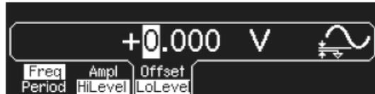
Note that these settings (high-level = "1.0 V" and low-level = "0.0 V") are equivalent to setting an amplitude of "1.0 Vpp" and an offset of "500 mVdc".
