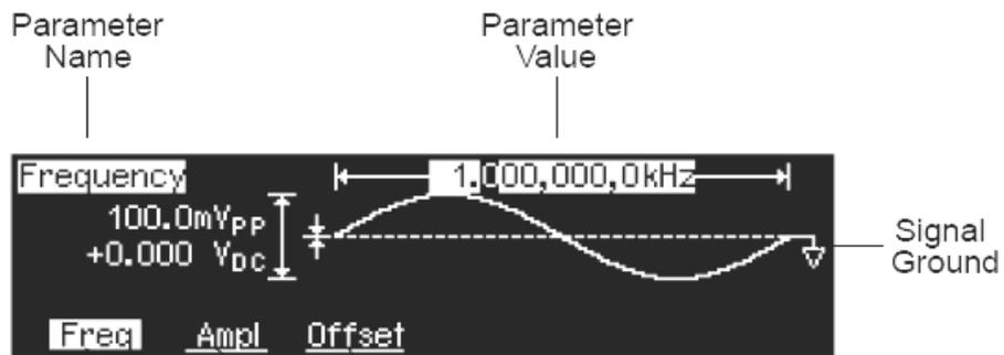
In Graph Mode, only one parameter label is displayed for each key at one time.
