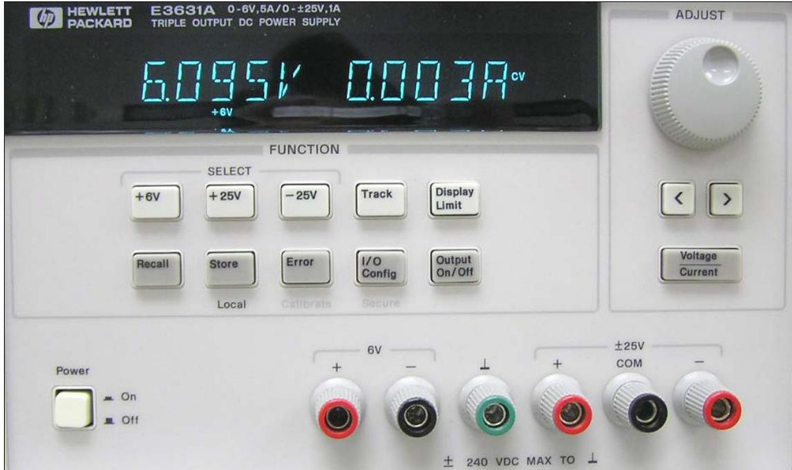
Figure 4: Front panel of the HP E3631A triple output power supply.
