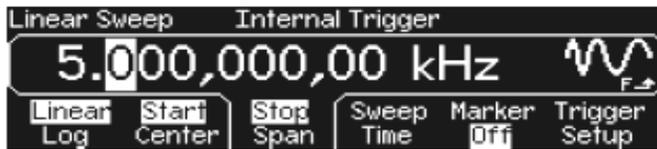
*At this point, the function generator outputs a continuous sweep from 50 Hz to 5 kHz (if the output is enabled).*
