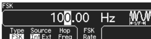
*At this point, the function generator outputs an FSK waveform (if the output is enabled).*
