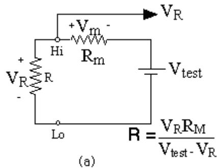
Figure 2: Two-wire resistance measurement
