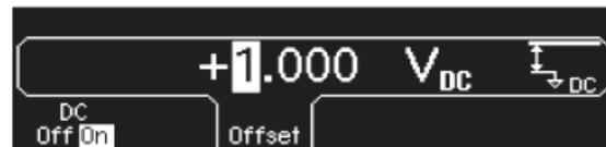
You can enter any dc voltage from -5 Vdc to +5 Vdc.
