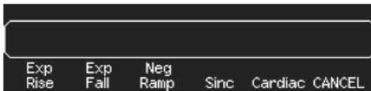
The selected waveform is now assigned to the **Arb** key. Whenever you press this key, the selected arbitrary waveform is output. To quickly determine which arbitrary waveform is currently selected, press **Arb**.
