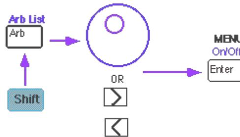
Figure 9: Selecting the Arbitrary Functions by pressing the SHIFT and ARB LIST keys
