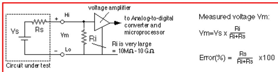
Figure 7: Schematic of the DMM as a DC voltage meter.
