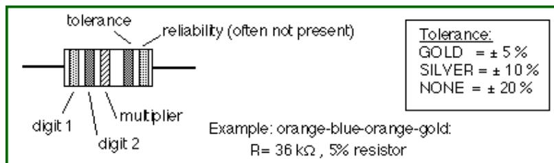
Figure 6: The 5% Resistor Color Code.
