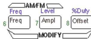
Figure 7: Using the Modify Keys to select the frequency, amplitude, offset or duty cycle
