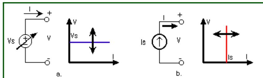
Figure 1: Output characteristic of a constant-voltage (a) and constant-current (b) supply.
