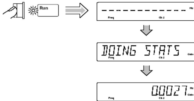
In this case, the displayed standard deviation value is computed on all measurements of the 10 MHz signal since no limits were set.
