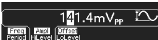
To change the displayed amplitude by *decades*, press the right-cursor key to move the cursor to the units on the right side of the display. Then, rotate the knob to increase or decrease the displayed amplitude by decades.
