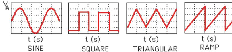
Figure 1: Waveforms generated by a function generator
