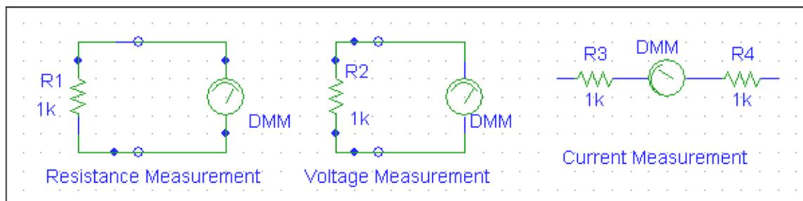
Figure 1: Measurement of resistance, voltage and current with a multimeter
