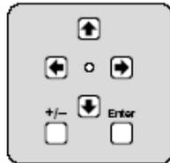
Press any one of these arrow keys to toggle to the next state of Auto Trigger.
