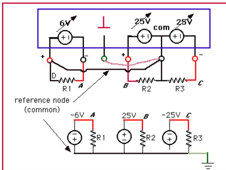
Figure 6: Power supply connection using the three power supplies; the top figure shows the actual connection and the bottom one gives the circuit schematic.
