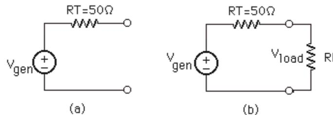
Figure 4: (a) Thevenin's equivalent circuit; (b) voltage divider between the output and load resistors.
