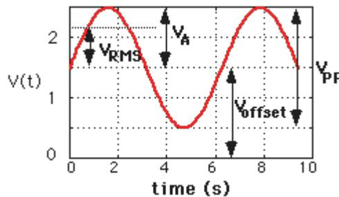
Figure 2: Sine wave with amplitude  $V_A$ , frequency  $f$ , and offset  $V_{\text{OFF}}$
