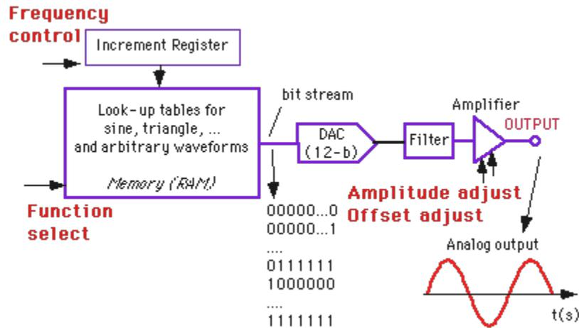
Figure 3: Block diagram of the HP33120A waveform generator.
