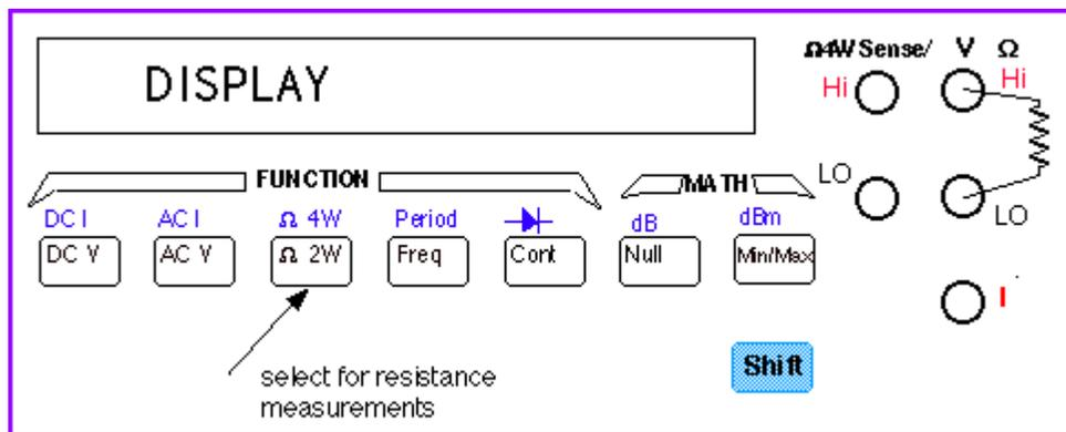
Figure 3: Function buttons to select resistance, voltage, current or frequency
