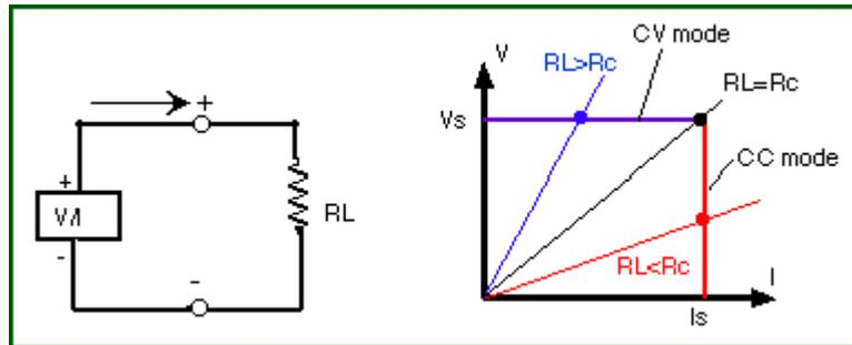
Figure 3: Operating point of a CV/CC power supply.
